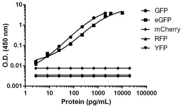
**Figure 3.** This kit recognizes both GFP and enhanced GFP (eGFP) in cell and tissue extracts. No reactivity with mCherry, RFP or YFP was observed.
