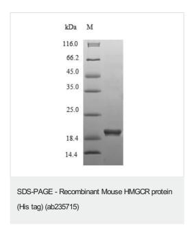
(Tris-glycine gel) Discontinuous SDS-PAGE (reduced) with 5% enrichment gel and 15% separation gel of ab235715.
