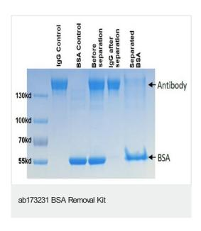
SDS-PAGE Gel showing the use of ab173231 BSA Removal Kit on a mixture containing 1 mg/ml lgG and 1 mg/ml BSA. The gel shows the mix before and after separation. 4-12% Bis-Tris gel, non-reducing.
