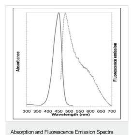
Absorption and fluorescence emission spectra for Green Detection Reagent dye. Spectrum was determined in 1X Assay Buffer.
