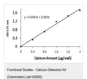
Example of standard curve obtained using ab102505
