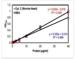
Typical absorbance plot obtained for BSA and Cytochrome C from Bovine Heart by using test tube procedure (60°C for 1 hour).
