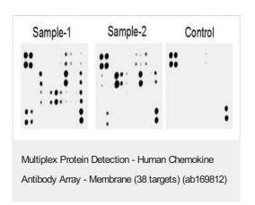
Typical images obtained with Abcam Human Cytokine Antibody Array. These membranes were probed with conditioned media from two different cell lines. Membranes were exposed to film at room temperature for 1 minute.
