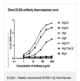
Direct ELISA antibody dose-response curve using ab125909 between 0-1000 ng/mL. Antigen concentration of 1000 ng/mL. An alkaline phosphatase-conjugated goat anti-rabbit lgG (H+L) (1/2500) was used as the secondary antibody.
