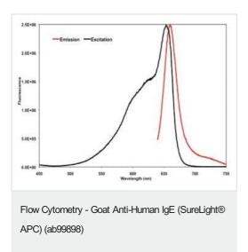
Fluorescence excitation and emission spectra of Allophycocyanin in 100mM sodium phosphate (pH7.2) + 1mM EDTA and 1mM sodium azide. The emission scan was taken with excitation at 630nm. The excitation scan was taken with an emission at 660nm. The curves were normailized to equalize peak heights.
