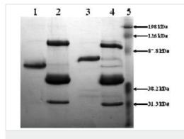
10% SDS-PAGE showing ab92728 Lane 1 ab92728 Non-reduced (3µg) Lane 2 ab92728 (3µg) + PAI-1 (12µg) Non-reduced Lane 3 ab92728 Reduced (3µg) Lane 4 ab92728 (3µg) + PAI-1 (12µg) Reduced Lane 5 MWM
