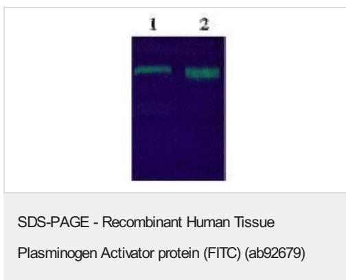
Staining of TPA Tissue Plasminogen Activator protein by 10% SDS-PAGE (UV trans-illuminator). Lane 1: ab92679 (3 µg) reduced Lane 2: ab92679 (3 µg) non-reduced
