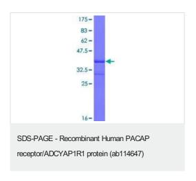
ab114647 analysed on a 12.5% SDS-PAGE gel stained with Coomassie Blue.
