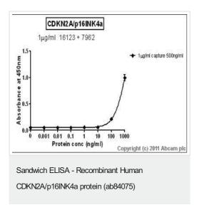
Standard Curve for CDKN2A/p16INK4a (Analyte: CDKN2A/p16INK4a protein (Human) (ab84075)); dilution range 1pg/ml to 1µg/ml using Capture Antibody Mouse monoclonal [DCS50.1] to CDKN2A/p16INK4a (ab16123) at 1µg/ml and Detector Antibody Rabbit polyclonal to CDKN2A/p16INK4a (ab7962) at 0.5µg/ml.
