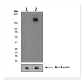
Western blot - Anti-EGFR (phospho Y1086) antibody [EP2258IHCY] (ab68470) **All lanes :** Anti-EGFR (phospho Y1086) antibody [EP2258IHCY] (ab68470) at 1/5000 dilution
