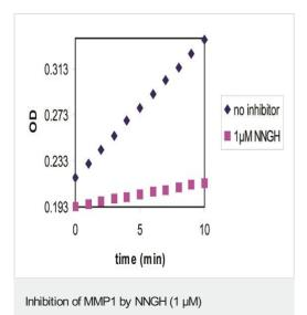
control slope = 1.20E-02 OD/min
