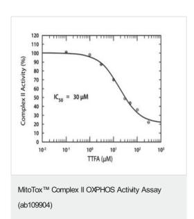
Typical dose response curve for TTFA (2-thenoyltrifluoracetone). Assay was performed following the Dose Response Assay Procedure using TTFA, a well known Complex II inhibitor. TTFA was prepared in DMSO to generate a 100 mM stock. Starting with a 500  $\mu$ M final concentration in well, 1:2 serial dilutions of TTFA were generated.
